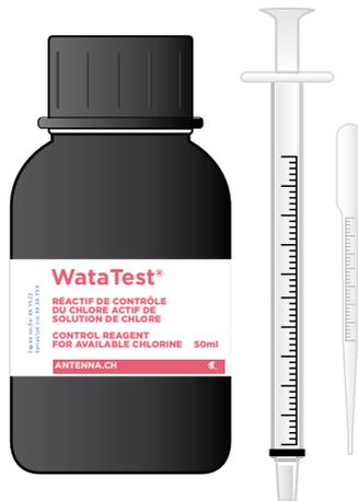
It is essential to test the quality of the sodium hypochlorite solution produced in order to determine the dosage to apply depending on its use.
