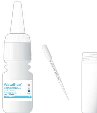
The WataBlue<sup>®</sup> reagent test determines the concentration of residual chlorine in the treated water.
