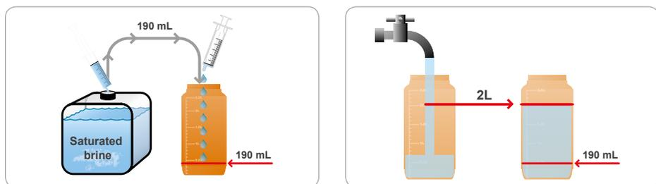
Using the large syringe (50 mL, supplied in the kit), inject **190 mL of saturated brine for 2 L of water to be electrolysed**, then top up your container using clean water (total volume 2 L).
