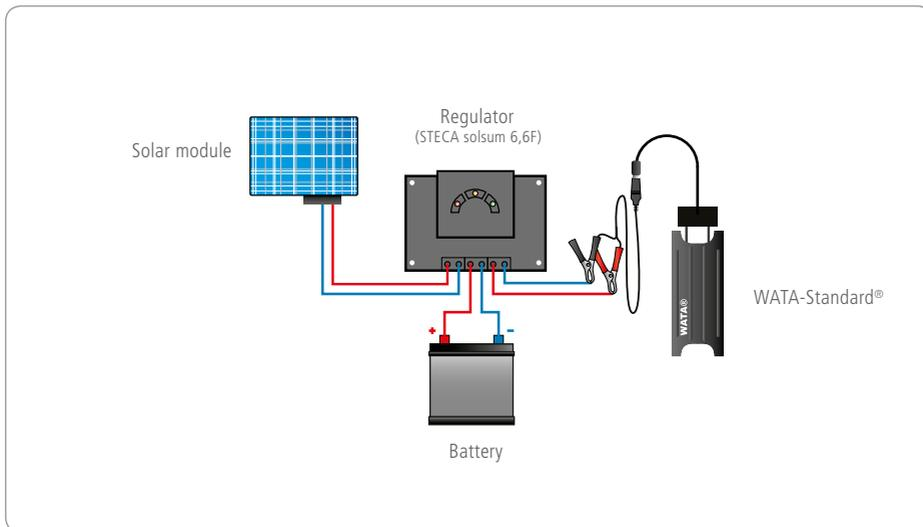
To determine the size of your solar module (solar electric panel, battery and regulator), we recommend that you consult a specialist. To give an idea of what is required, the tables below show approximately the capacity of the battery and peak power of the solar panel that are necessary depending on your needs and on the amount of solar radiation.
