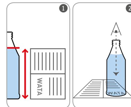
⚠️ There should be ample illumination but the light should not be blinding. The bottle should be transparent, colourless, clear and without scratches or dirt. A flat-bottomed bottle is preferable. Since it is not always possible to meet all of these conditions, catching a slight glimpse of the WATA® logo is acceptable.
