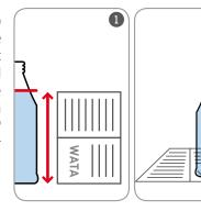
A There should be ample illumination but the light should not be blinding. The bottle should be transparent, colourless, clear and without scratches or dirt. A flatbottomed bottle is preferable. Since it is not always possible to meet all of these conditions, catching a slight glimpse of the WATA® logo is acceptable.
